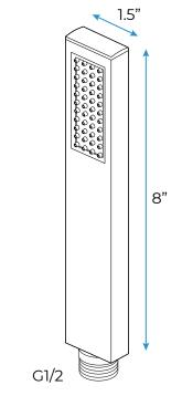
Flow Rate: 2.0 GPM / 7.6 LPM
